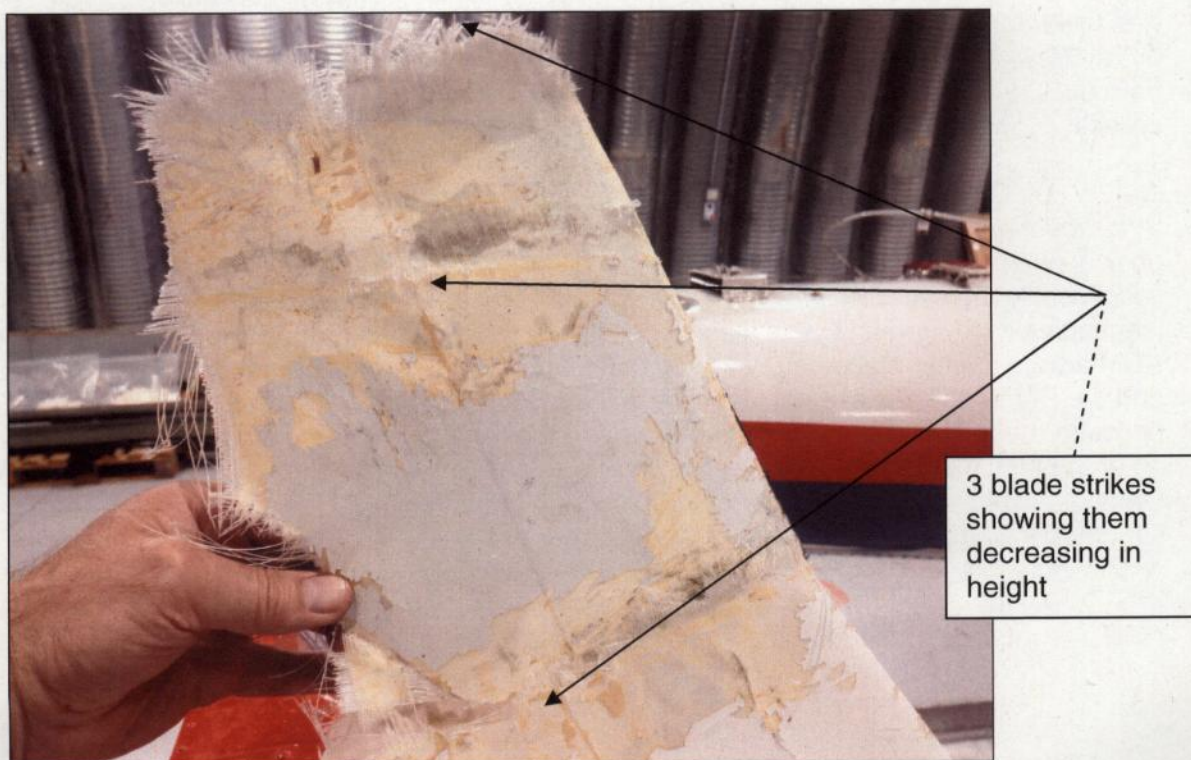
Fig 4 - Blade interaction with Lateral Stabilizer
