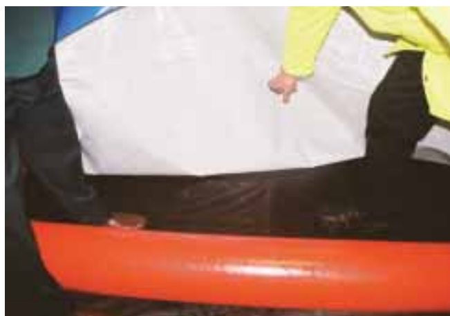
Photograph 6: A leaking chemical liner in a mobile decontamination unit.
