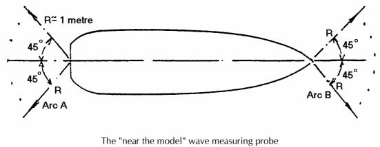
to be positioned either on arc A or arc B
