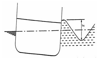
1. If  $h_s \ge 4.0$  metres, height of water on deck is calculated as per figure 3
