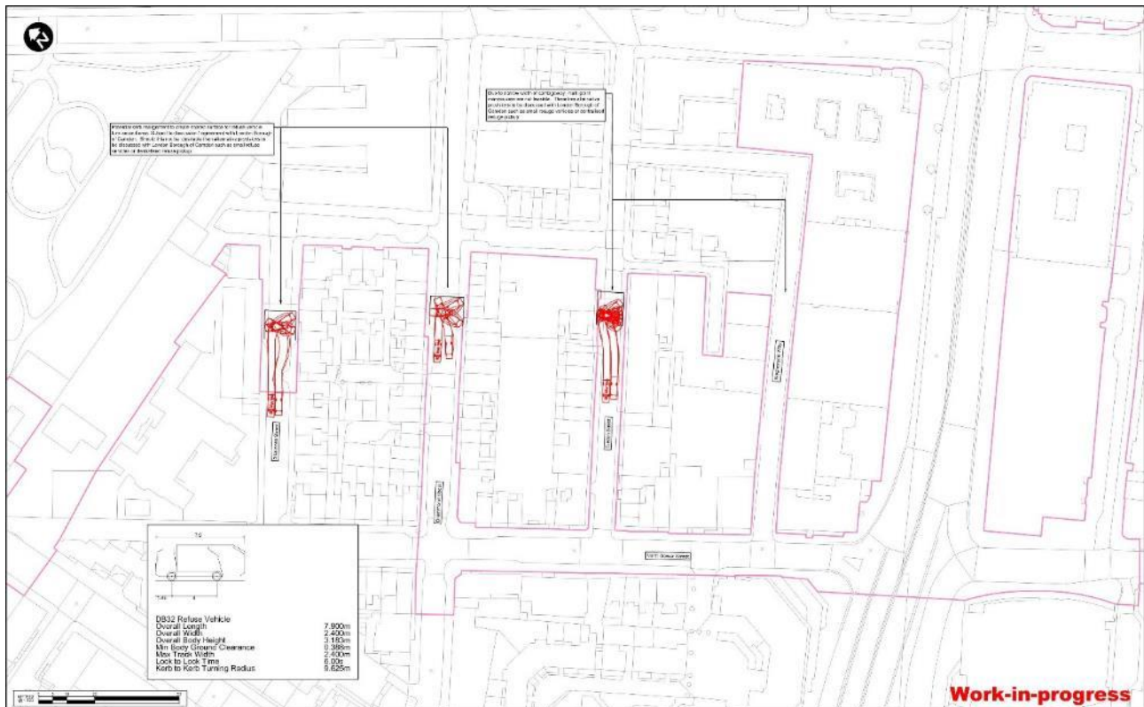
Figure 108: Refuse collection vehicle access on Starcross Street, Drummond Street and Euston Street
