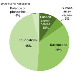
Figure 5.1 Breakdown of balance of plant supply costs.
