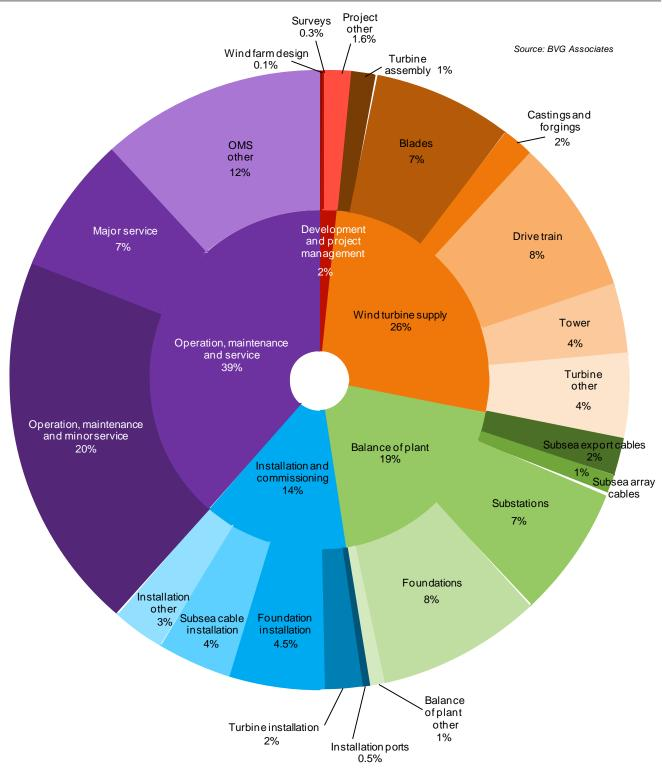
Figure 2.2 Breakdown of undiscounted capital and operational costs of a typical offshore wind farm. These are based on a 500MW wind farm using 6MW turbines and jacket foundations using a combination of real project and modelled data. In some cases percentages have been rounded to fewer significant figures than those in the main text of the report.
