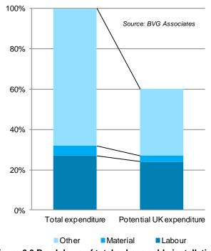
Figure 6.6 Breakdown of total subsea cable installation expenditure and potential UK expenditure.
