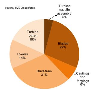
Figure 4.1 Breakdown of turbine supply costs. Based on a 6MW turbine with 147m rotor
