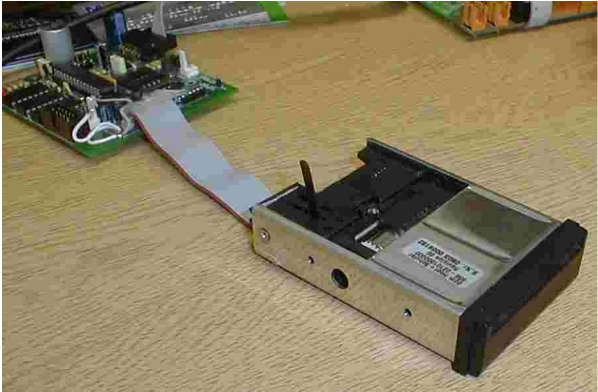
Figure 17 Hopt and Schuler MCR combined smart-card and magnetic stripe reader/writer
