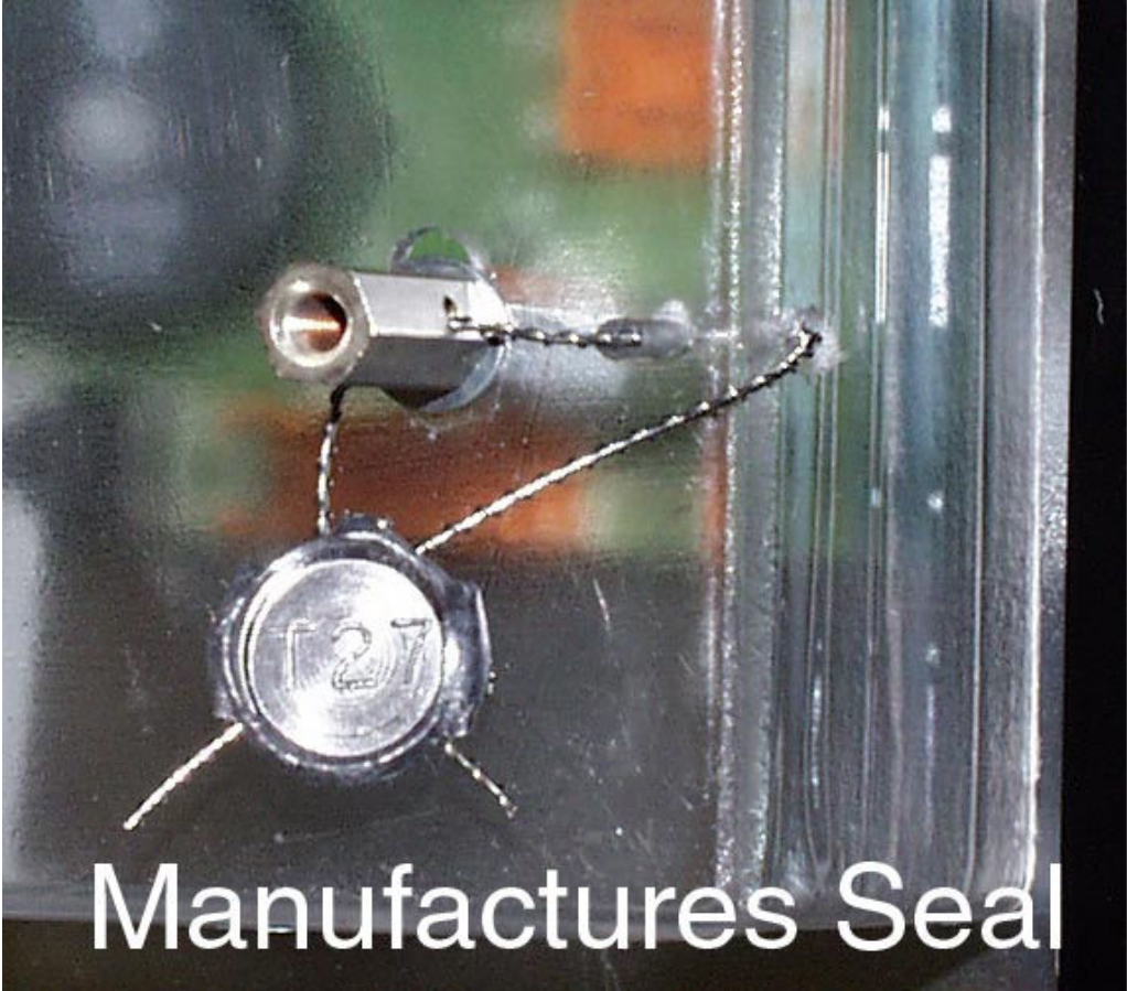
Figure 6 View showing manufacturer's sealing arrangement for the PC board cover
