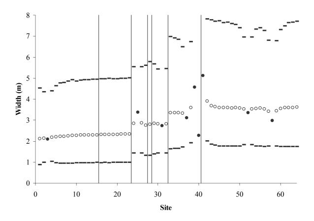
Figure 4.4 Estimated widths for Nant-y-Goron, River Conwy. Closed circles denote width measurements, and open circles denote width estimates. Horizontal lines give upper and lower 95% confidence intervals. Vertical lines denote confluences.
