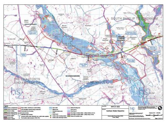
Surface Water Baseline Plans show the proposed scheme's alignment in relation to existing surface water features and areas at varying risks of flooding.
