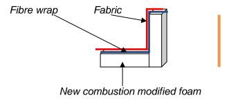
3. Essentially, these changes make the test set-up a closer approximation of an actual piece of furniture. Now, because cover fabrics will not need to carry the full burden of acting as a barrier to ignition, less FRs will be required.
