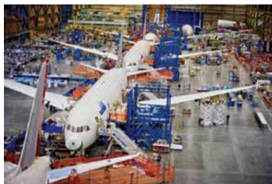
Figure 7: Boeing 787 Assembly facility showing limited use of tooling. (Photograph reproduced with kind permission of the Boeing Company).
