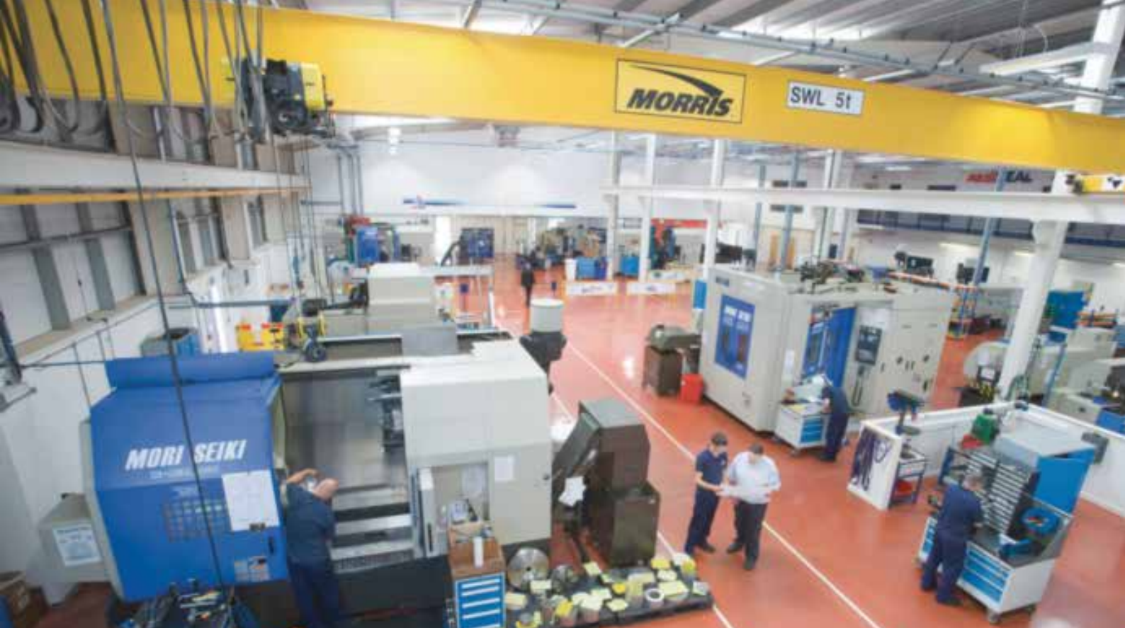
Figure 1: The workshop environment, AES Seals Ltd, Rotherham showing many facets of the FoF. (Lean, clean, bright, reconfigurable, CNC machine tools grouped in flexible cells). Photograph reproduced with kind permission of AES Seals Ltd, Rotherham.
