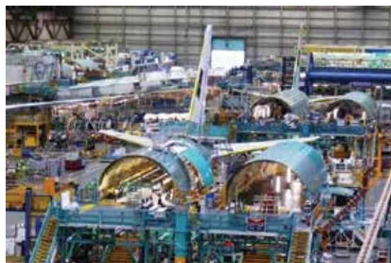
Figure 8: Traditional aircraft assembly facility (Boeing 767) showing the dependence on large tooling facilities (Photograph reproduced with kind permission of the Boeing Company).
