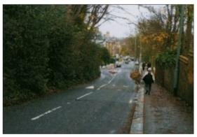
Photo 3.7.1: Mini-roundabout on hill descent with speed reducing measures on approach
