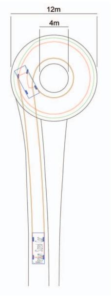
Figure 3.3: Sample Desirable Minimum ICD
