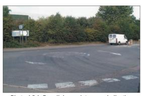
Photo 4.5.1: Poor lining maintenance indicating frequent central island overrunning
