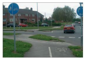
Photo 3.11.2: Mini-roundabout with off-highway cycle facilities
