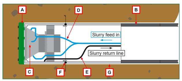
Figure D1: Schematic of a slurry shield TBM
