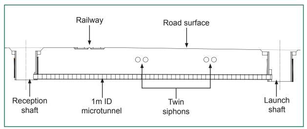
Figure 7: Schematic cross-section through microtunnel and construction shafts
