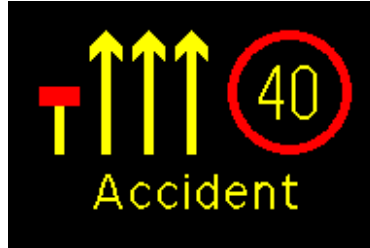
Figure 4G: Variable Message Sign warning of a closed lane ahead due to an accident
