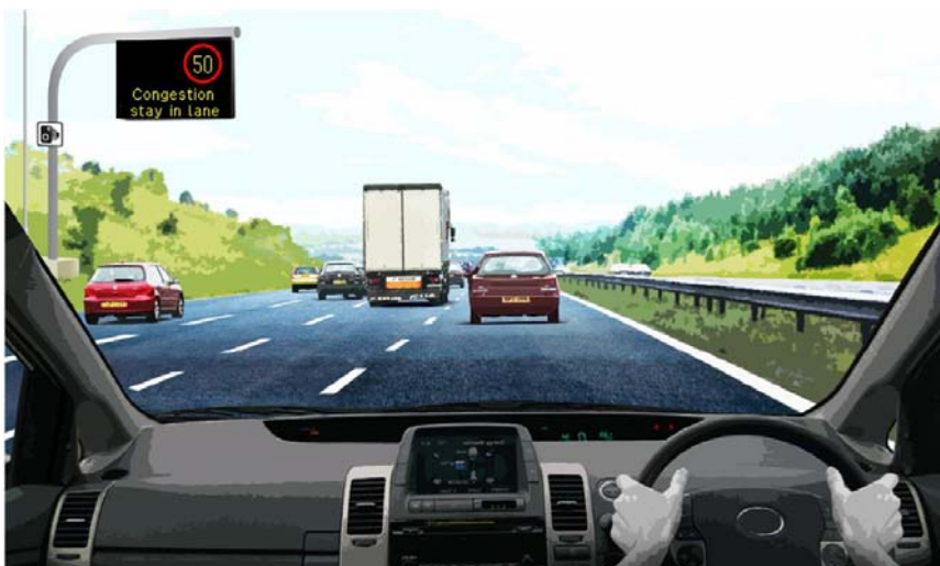
Figure 4C: Illustrative M3MM section operating with Variable Mandatory Speed Limits
