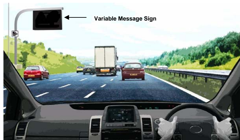
Figure 4B: Illustrative M3MM section operating in normal motorway conditions with a blank verge mounted Variable Message Sign
