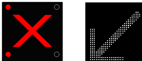
Figure 4E: Red X (STOP) aspect with flashing red lanterns and a lane divert signal shown on an Advanced Motorway Indicator over any lane
