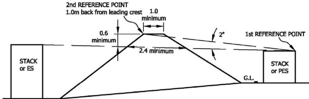
Figure 2 - Determination of Traverse Height on Sloping Terrain
