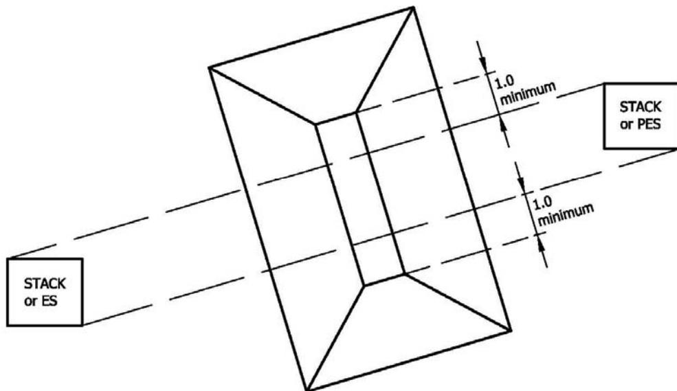
Figure 3 - Determination of Traverse Length
