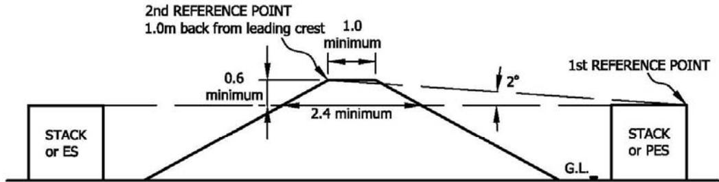
Figure 1 - Determination of Traverse Height on Level Terrain
