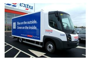
(Shiers, 2009). Modec vehicles also allow customisation according to customers' needs. For example, Tesco vans are fitted with refrigeration technologies that do not draw on electric current (What Van, 2008).
