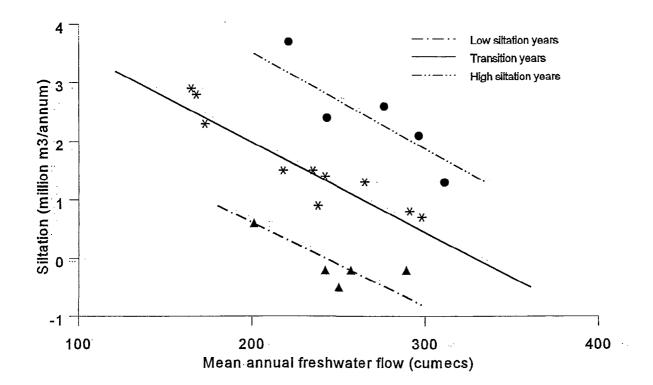
Figure 1.1 - SUNK DREDGED CHANNEL - RELATIONSHIP BETWEEN MEAN ANNUAL FRESHWATER FLOW AND ANNUAL SILTATION
