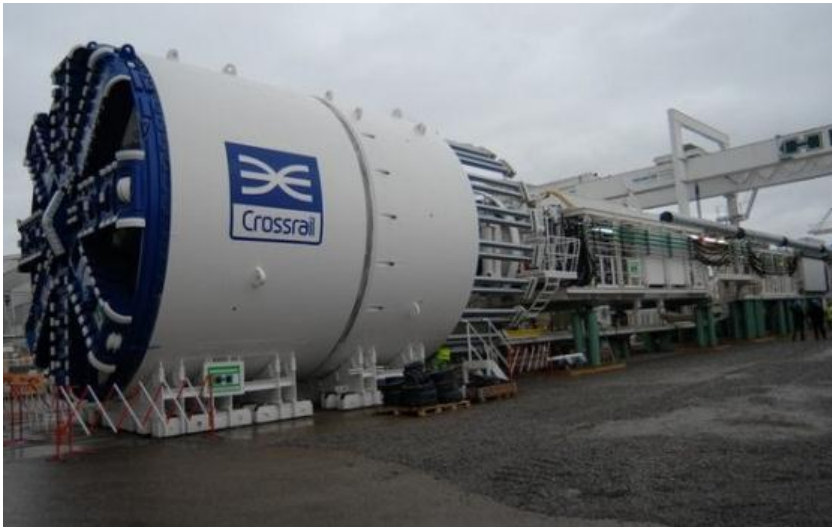
Tunnel Boring Machine
