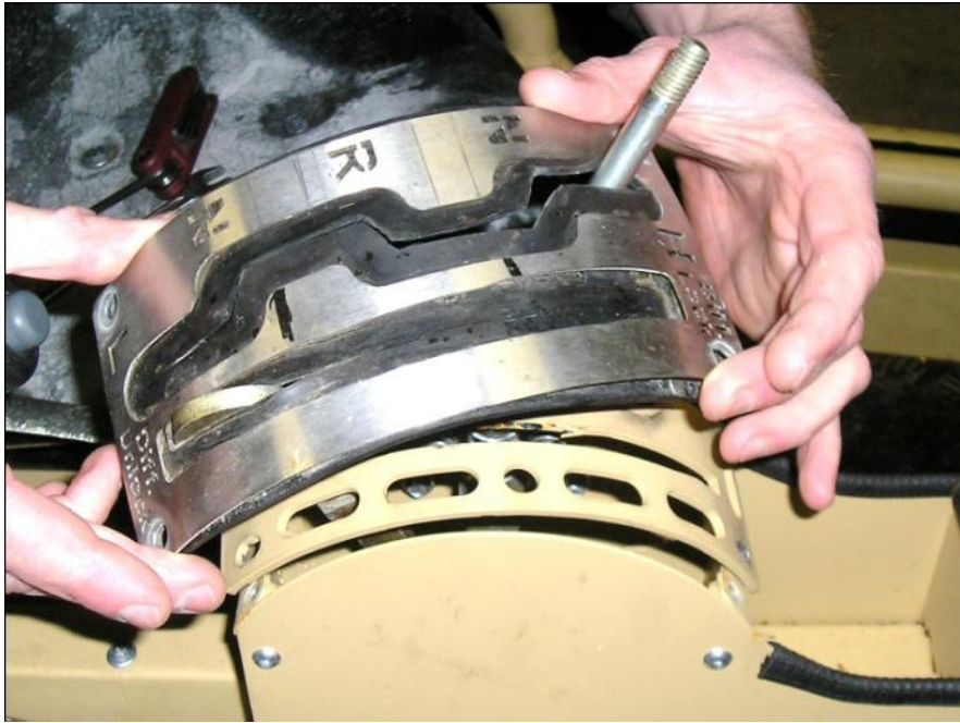
Fig 1 Removal of Gear selector Plate
