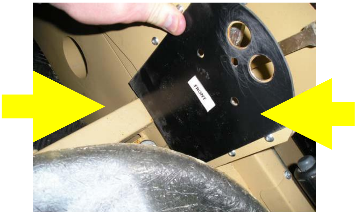
Fig 3 Fitting of Template – Ensure that the template is lined up between the M6 Bolt heads as shown
