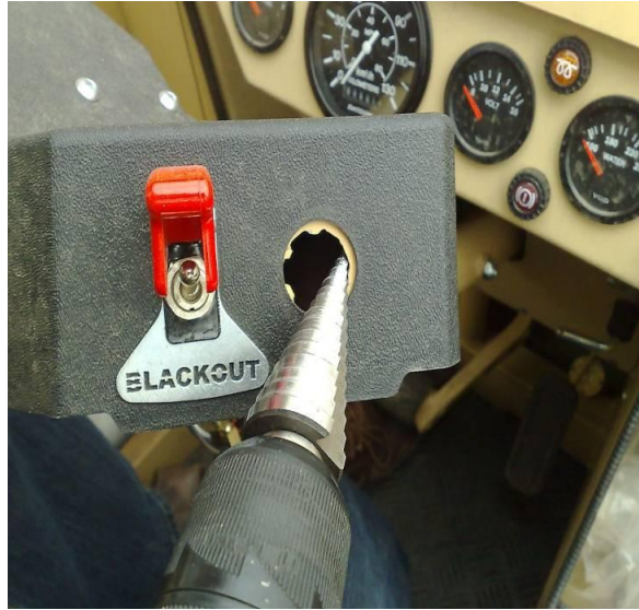
Fig 2 Drill out the fitting hole to 22mm
