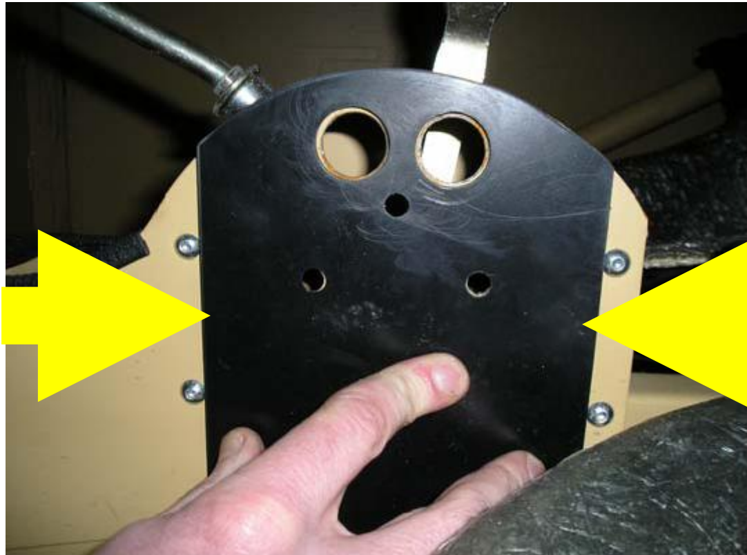
Fig 3 Fitting of Template – Ensure that the template is lined up between the M6 Bolt heads as shown
