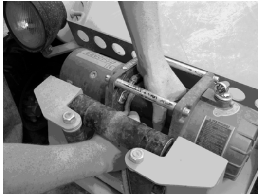
Fig 9 Manually turn the winch drum
