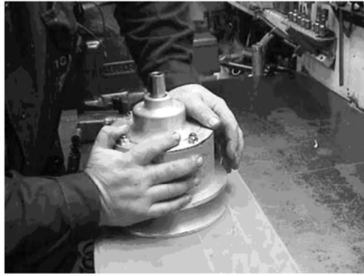
Fig 4 Engine CVT inspection
