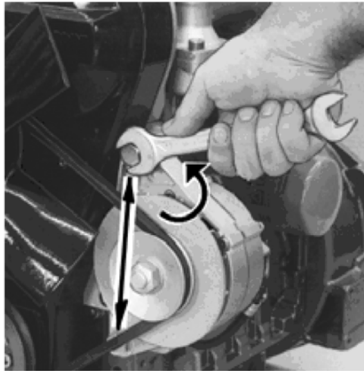
Fig 38 Alternator mounting bolts
