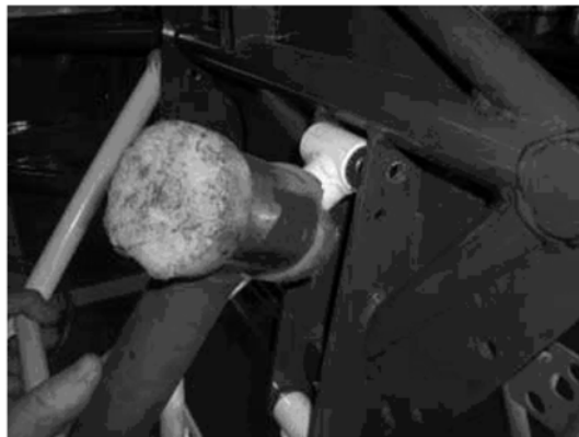
Fig 35 Install the A-arm to the chassis
