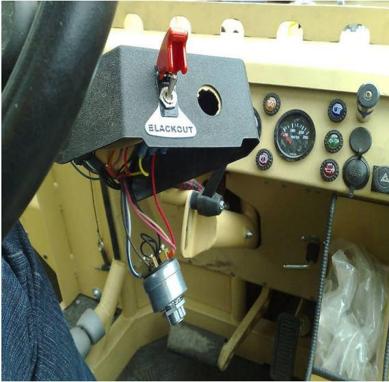
Fig 1 Remove Old Ignition Switch
