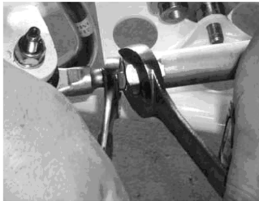
Fig 12 Adjust the toe-in
