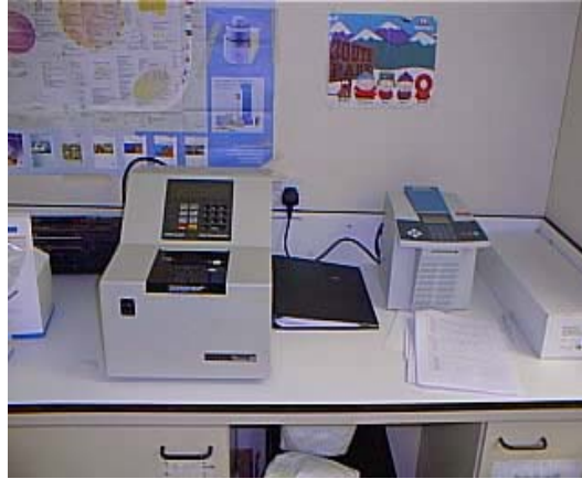
Figure 2.2 Two PCR machine suitable for routine amplification of nucleic acids
