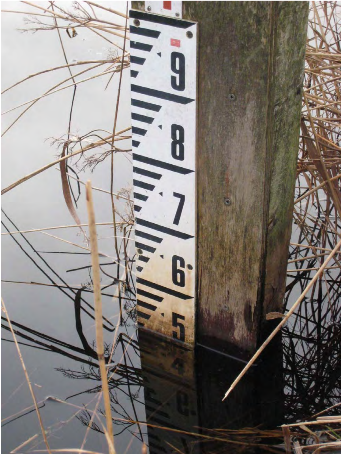
Figure J3 Gaugeboard NTG3261G1 within the internal system, close to the northern sluice. Note iron staining on the gaugeboard extends up to the 6.5 mark (27/2/2012)
