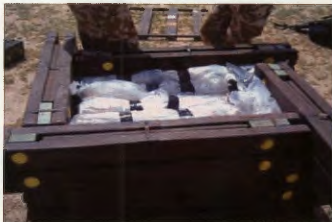
Fig. 2 (right): Canister placed in barmine stack. Further barmines were then placed over the 'lid' and donor charges and initiators fixed.
