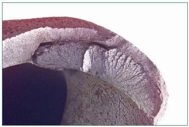
*Figure 14: Cracking from the inside of one corner after corrosion removal (photograph courtesy of Serco Technical & Assurance Services, Derby)*
