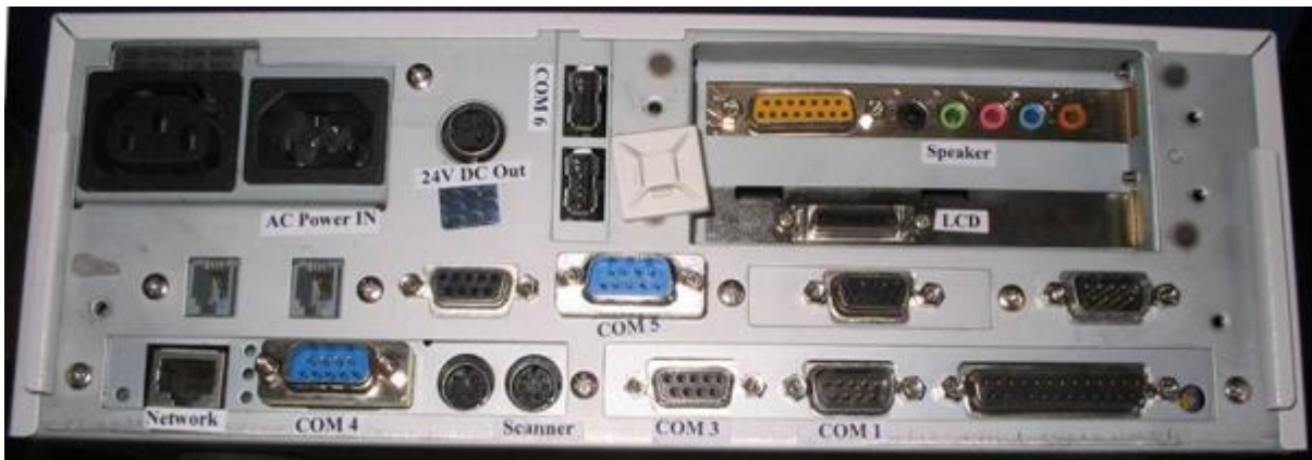
Figure 33 Toshiba TEC ST-6501, schematic view showing ports and connections – cover removed
