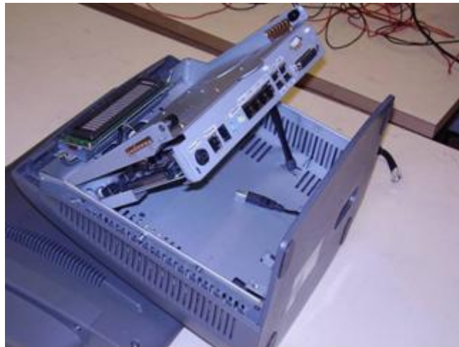
Figure 36 Aures Galeo POS PC showing ports and connections – cover removed
