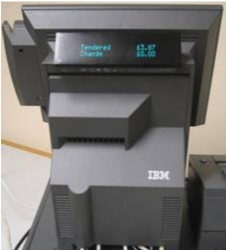
Figure 23 IBM surePOS 563, rear view showing integrated CDU
