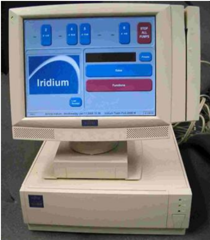
Figure 28 Fujitsu team POS 2000-M, showing integrated card swipe
