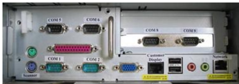
Figure 27 Epson IR 700 / IM 700 – showing rear connections with protective cover removed
