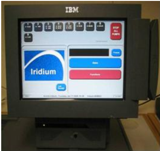
Figure 22 IBM surePOS 563, showing integrated card swipe
