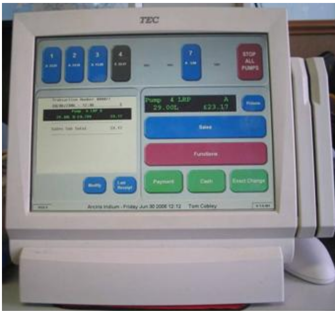
Figure 31 Toshiba TEC ST-6501 – TFTST56 flat display showing integrated card swipe
