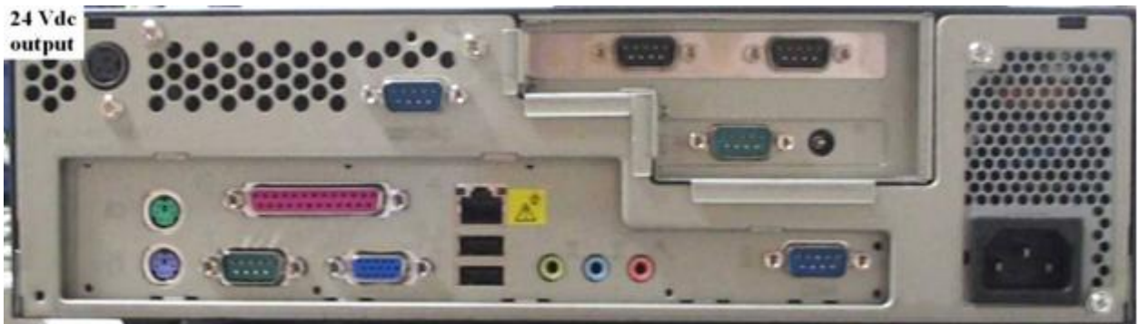
Figure 21 View of back panel – cover removed - showing 24 V outlet
