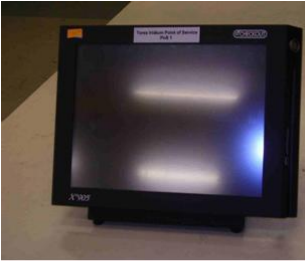
Figure 40 Xn905 POS PC (showing operator display)
