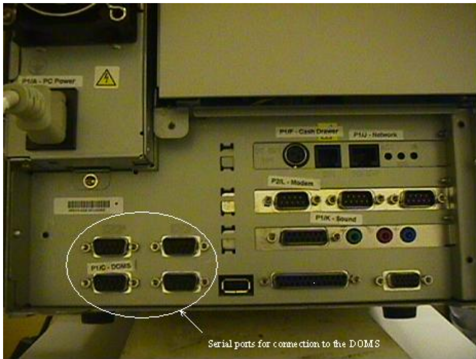
Figure 14 Rear of Epson IM-310 showing serial ports for connection to the DOMS
