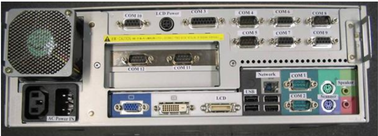
Figure 30 Fujitsu team POS 2000-M, schematic view showing ports and connections – cover removed
