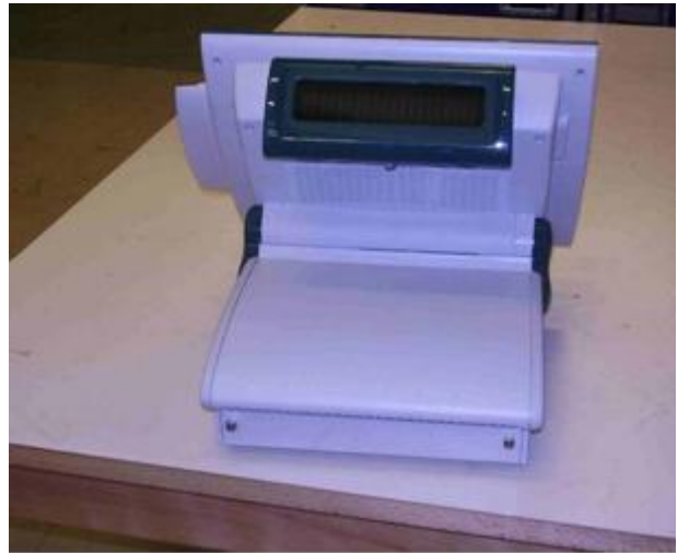
Figure 38 Aures Odysse POS PC (showing customer display)
