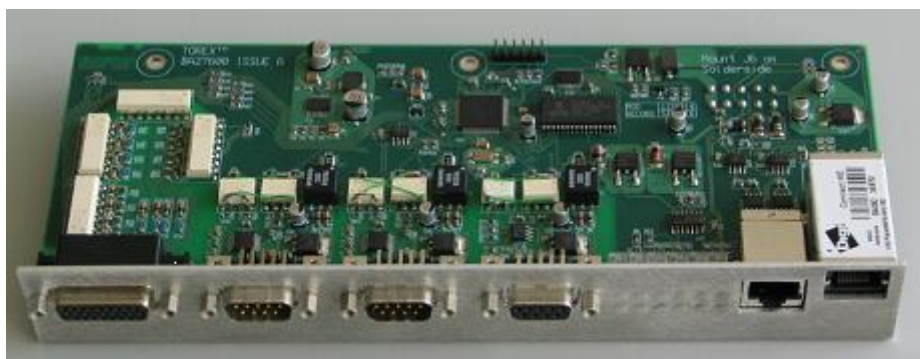
Figure 49 Forecourt Link Interface Box Control/PSU Board
