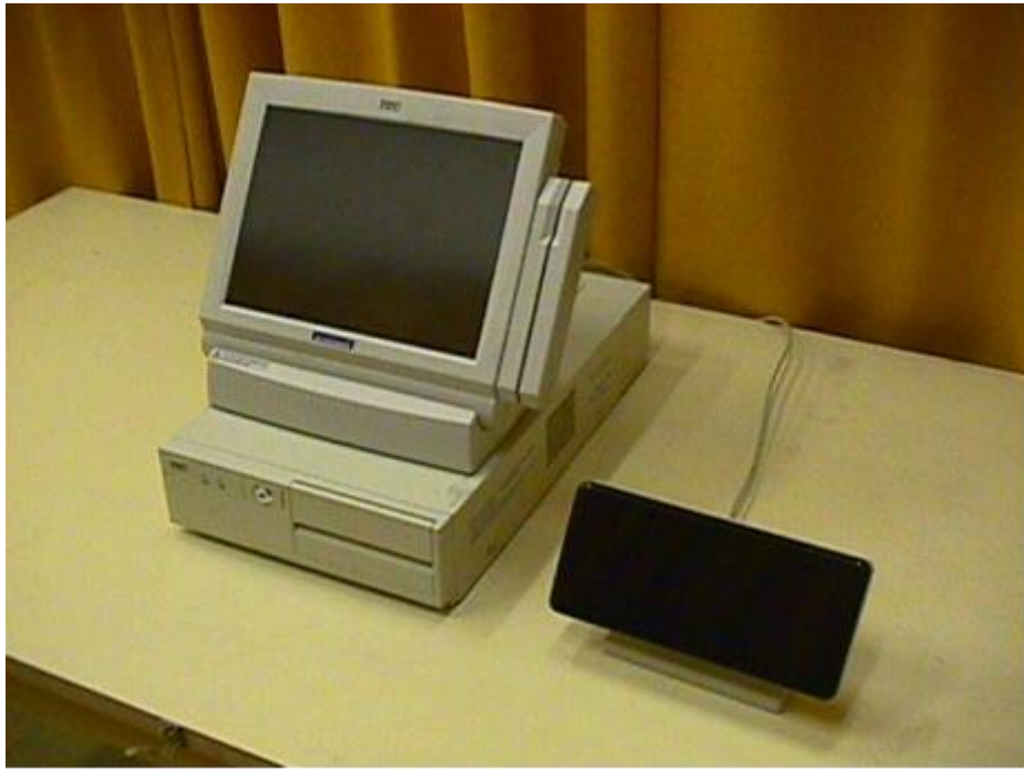
Figure 11 TEC 5600 POS system (PC with 2 expansion slots)
