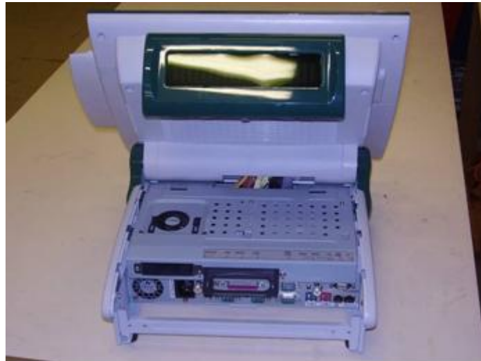
Figure 37 Aures Odysse POS PC (showing operator display)
