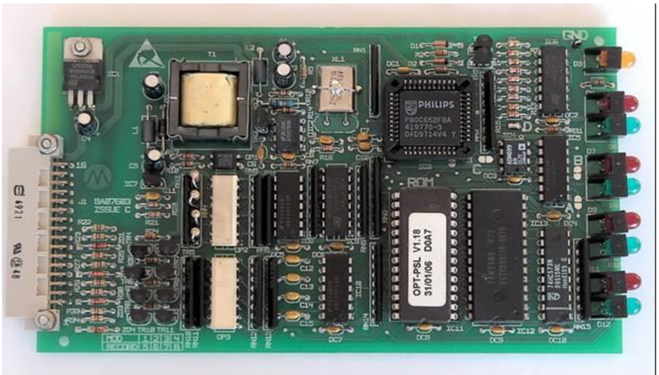
Figure 52 Torex Dispenser Interface Card type BA07603
