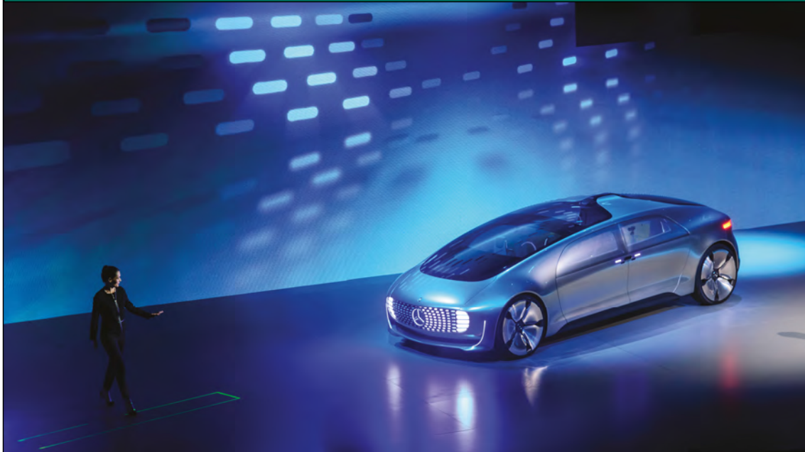
Figure 6.2 – The Mercedes F015 demonstrating its laser projected zebra crossing to help communicate with pedestrians that it is safe to cross
