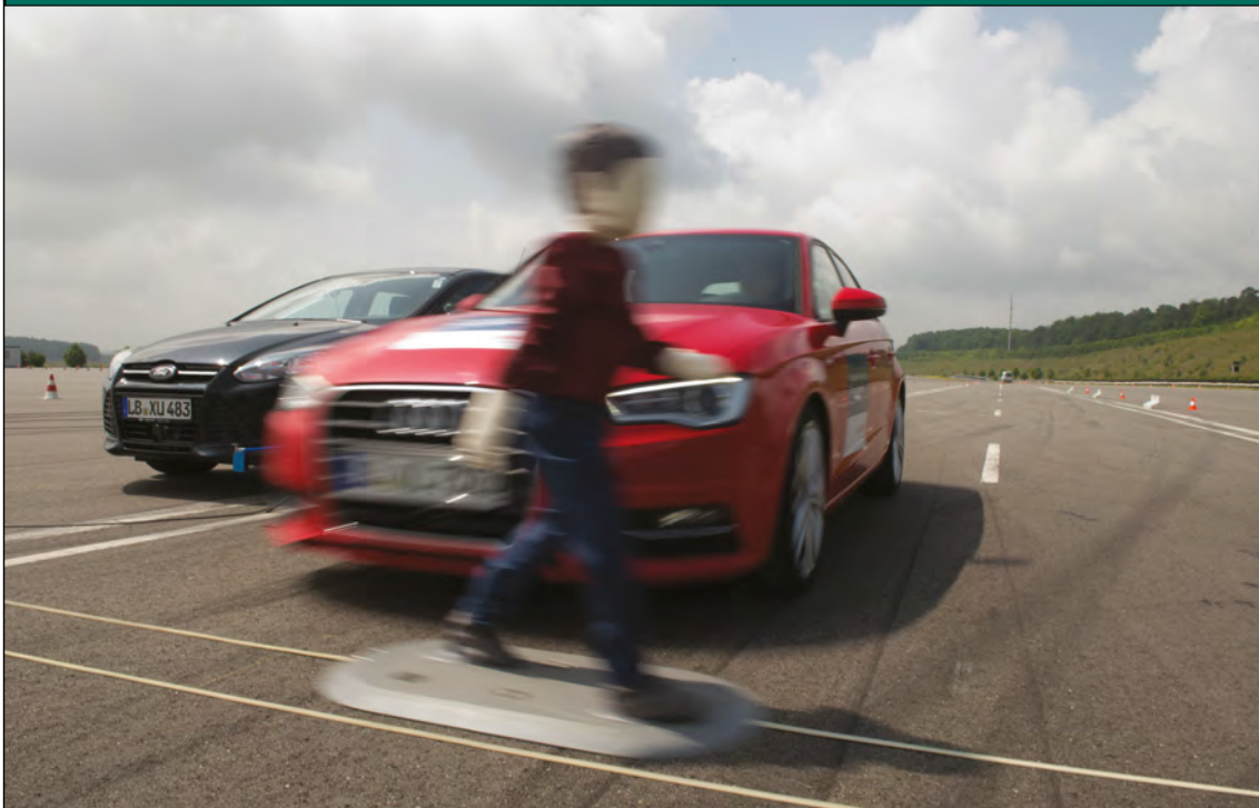
Figure 6.1 – Testing of automated braking system on private test track with child pedestrian dummy
