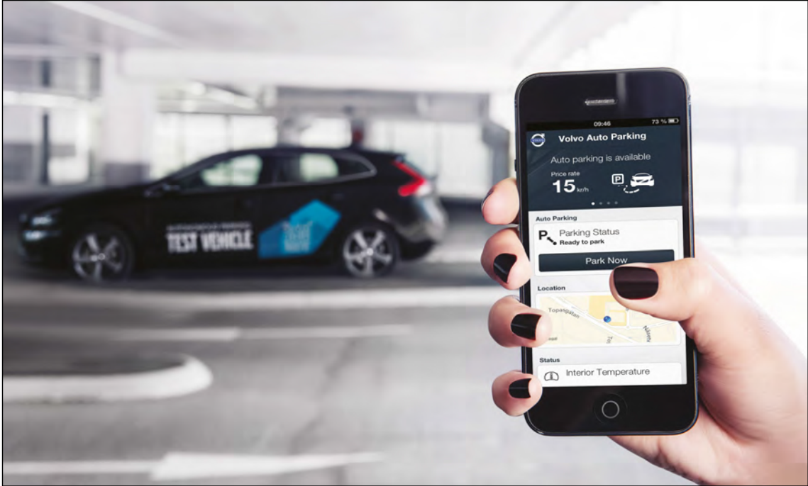
Figure 8.2 – Automated parking system, operated from a mobile phone application
