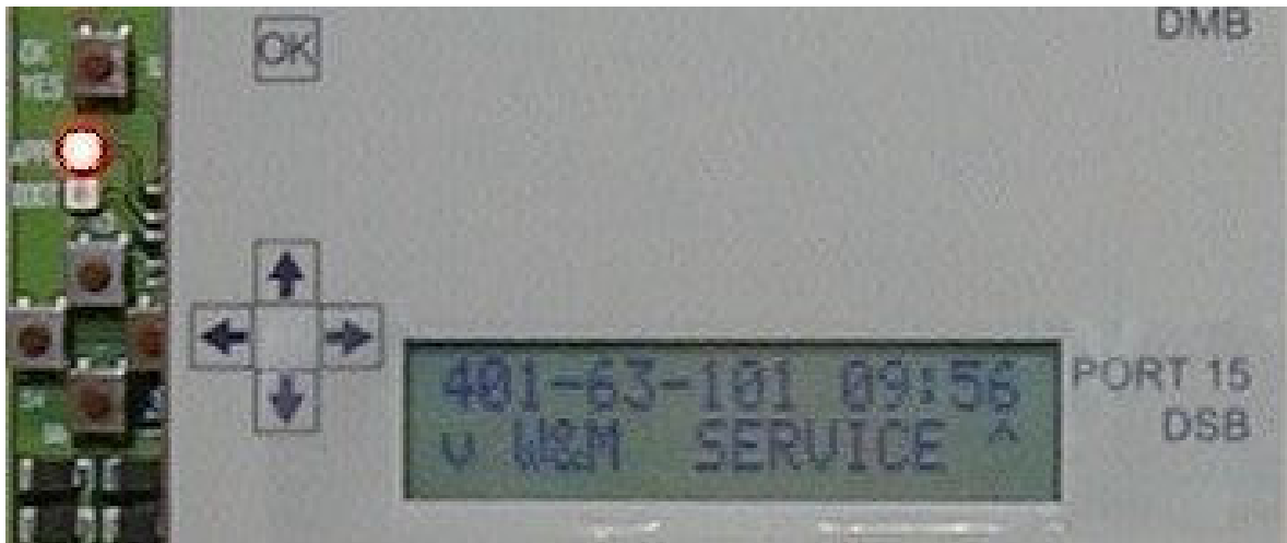
Figure 3 Central Processing Board (CPB508) display and menu navigation keys
