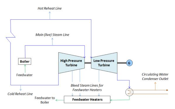
This example considers a typical small scale conventional steam plant with reheat, and a water cooled surface condenser. This is based on separate HP and LP steam turbines. The LP steam turbine could have a lateral or axial exhaust. There is no crossover pipe.
