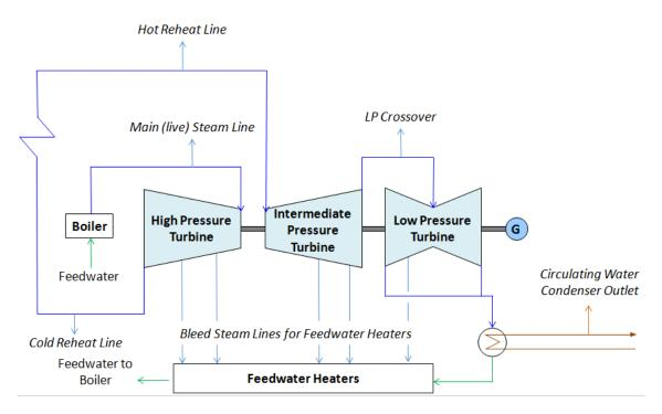
This example considers a typical large scale conventional steam plant with reheat, and a water cooled surface condenser. This is based on separate HP, IP and LP steam turbines. The LP steam turbine(s) have down exhausts, and the steam is delivered from the exhaust of the IP steam turbine to the LP steam turbine by large crossover pipes.
