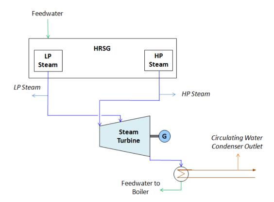
This example shows a typical small scale CCGT plant without reheat, and a water cooled surface condenser. This is based on a single case steam turbine with two pressures. The steam turbine could have a lateral or axial exhaust. There is no crossover pipe.
