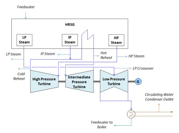
This example considers a typical large scale CCGT plant with a three pressure reheat, and a water cooled surface condenser. This is also based on separate HP, IP and LP steam turbines. The LP steam turbine(s) have down exhausts<sup>22</sup>, and the steam is delivered from the exhaust of the IP steam turbine to the LP steam turbine by large crossover pipes. There are usually no feedheaters, but multiple pressures are generated in the Heat Recovery Steam Generator (HRSG).
