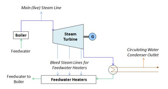
This example considers a typical small scale conventional steam plant without re-heat, and a water cooled surface condenser. This is based a single casing Steam Turbine. The Steam Turbine could have a lateral or axial exhaust. There is no crossover pipe.
