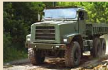
The Oshkosh MTVR has an off-road payload capacity of more than 6 tonnes and thrives in both on- and off-road environments.
