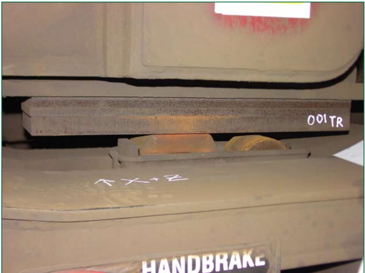
Figure 7: Photograph showing condition of a side bearer assembly
