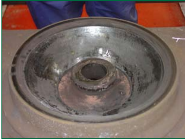
Figure 9: Condition of leading and trailing centre pivot socket liners
