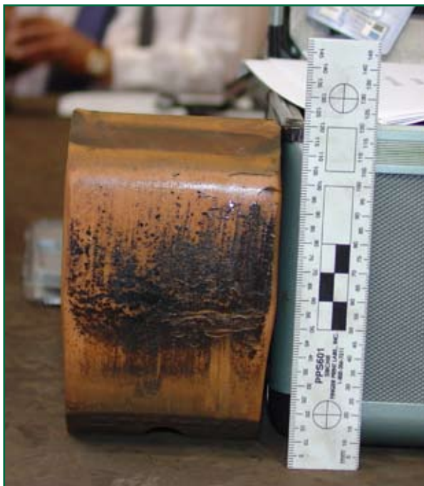
Figure 8: Condition of leading and trailing side bearer blocks
