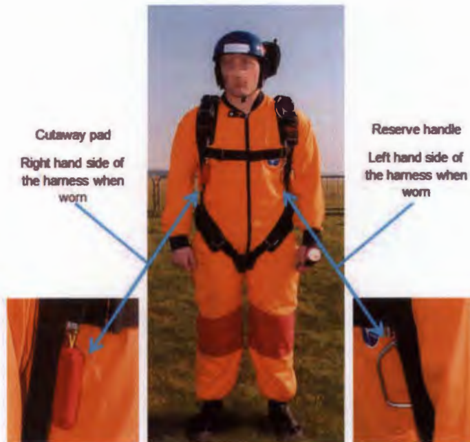
Fig 1.4.1 – Cut Away Pad and Reserve Handle Locations.
