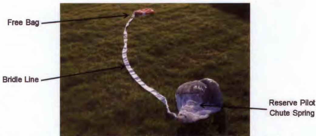
Fig 1.4.6 – LCpl Woodfords Reserve Pilot Chute Spring, Free Bag and Bridle Line.
