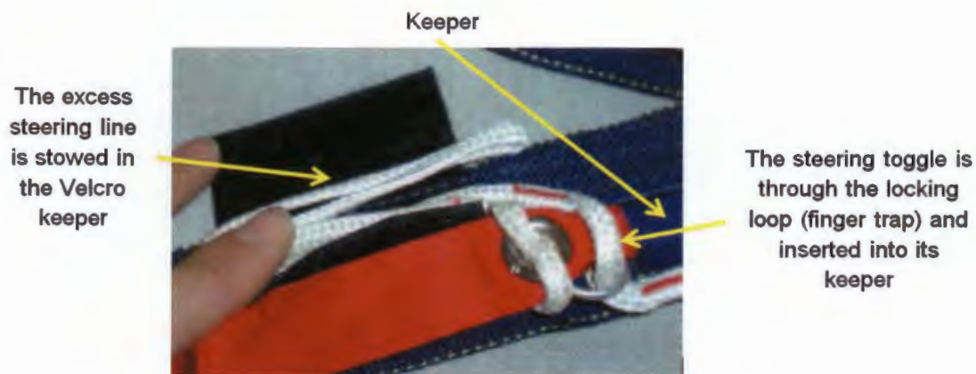
Fig 1.4.12 – Steering Toggle Set at Half Brake.
