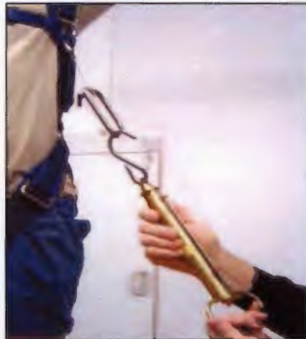
Fig 1.4.10 – Measuring the Reserve Handle Pull Off Tension.
