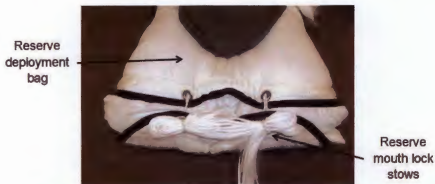
Fig 1.4.11 – Mouth Lock of the Reserve Deployment Bag.
