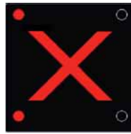
Figure 4E: Red X (STOP) aspect with flashing red lanterns and a lane divert signal shown on an Advanced Motorway Indicator over any lane
