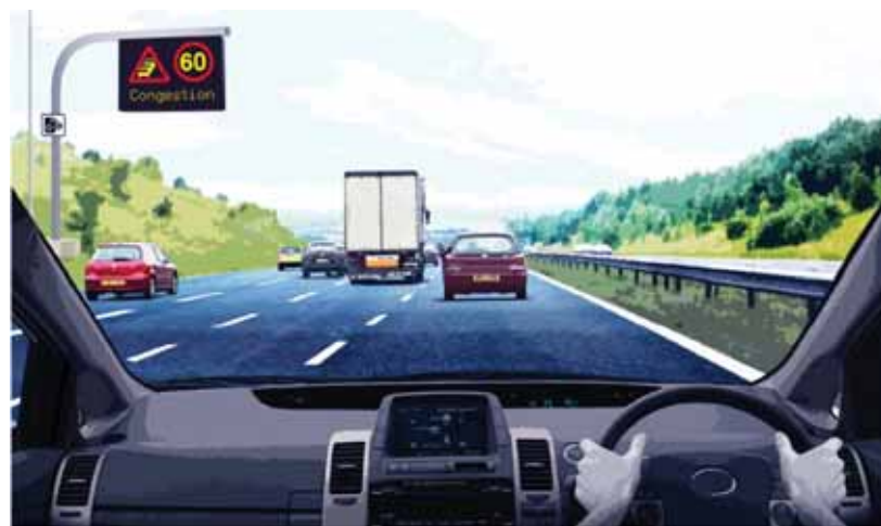
Figure 3D: Illustrative M25MM section operating with Variable Mandatory Speed Limits and information for road users
