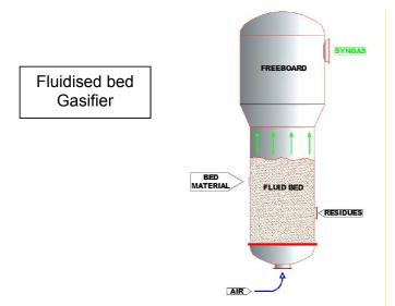
The gasifier requires air to fluidize the bed and to have the necessary oxygen for gasification reactions. The fluidisation air will be supplied by a compressor and will be uniformly distributed at the bottom of the reactor by an air distribution grill with nozzle type diffusers.
