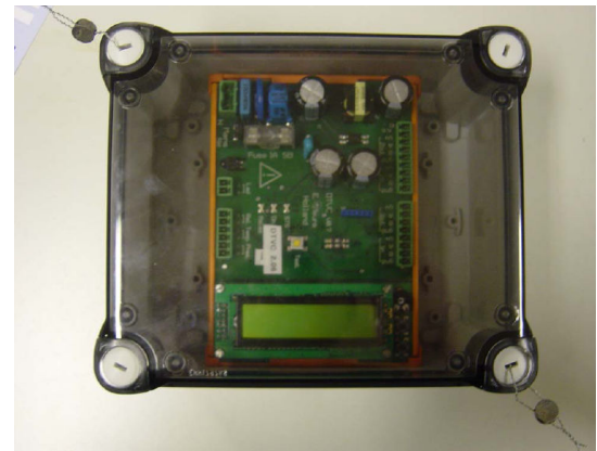
Figure 36 TVC unit sealing arrangement
