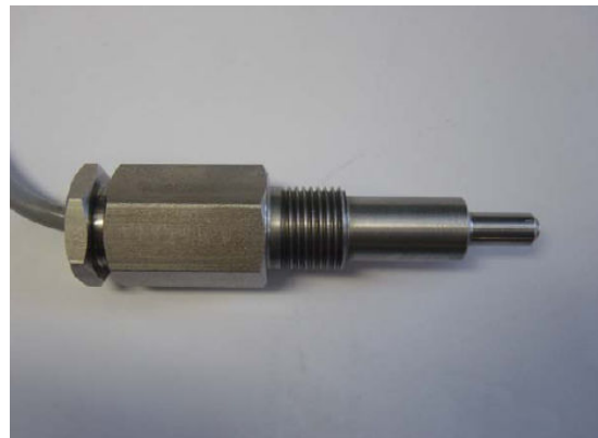
Figure 34 Temperature sensor: LM335
