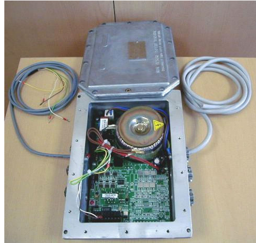
Figure 26 Nuovo Pignone Vapour recovery module (explosion proof version)
