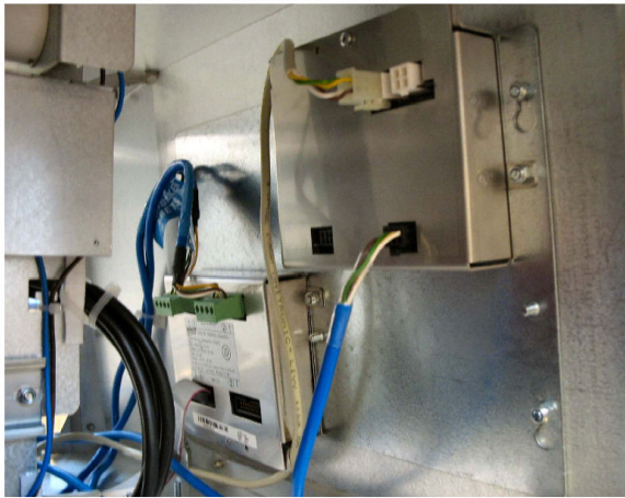
Figure 40 Dresser Wayne ATC – ISB mounted in electronic head
