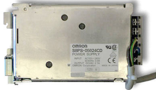
Figure 15 IGEM - Power supply unit
