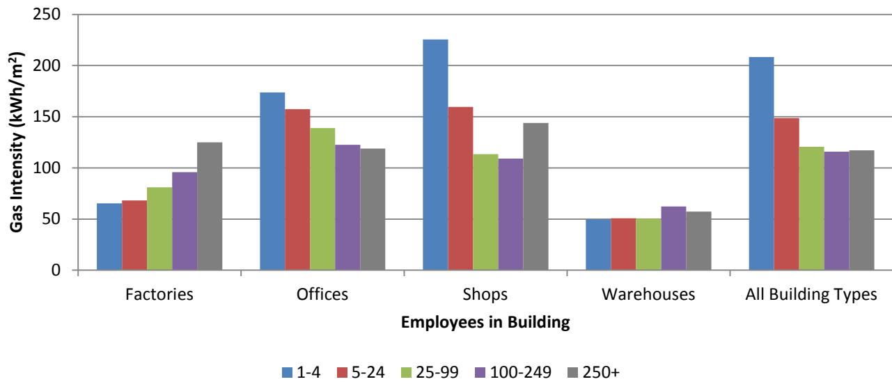
Figure 14: Median gas intensity by building type and by employee numbers, England and Wales, 2011.
