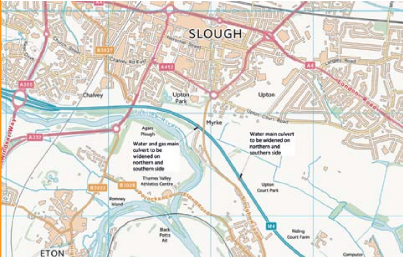
Figure 23: Service Culverts, Datchet
