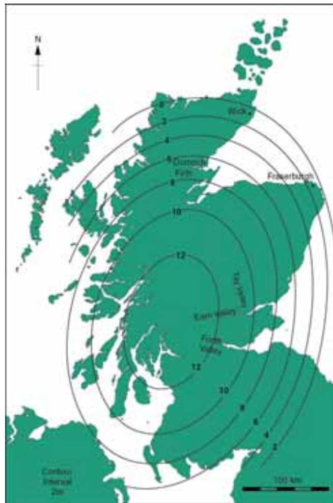
Figure 3 Isobases showing the uplift of the post-glacial shoreline on the Scottish mainland. Because the sea lochs penetrate so far inland it is possible to determine the uplift near the centre of the zone of isostatic uplift. (From Smith et al., 1999).
