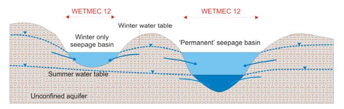
Figure 3.23 Schematic section of a Fluctuating Seepage Basin (WETMEC 12).
