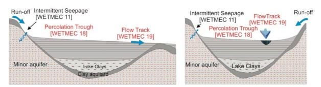
Figure 3.35 Schematic sections of types of Percolation Troughs (WETMEC 18) and Flow Tracks (WETMEC 19).
