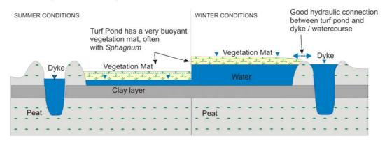
Figure 3.12 Schematic sections of Surface Water Percolation Floodplains (WETMEC 6).
