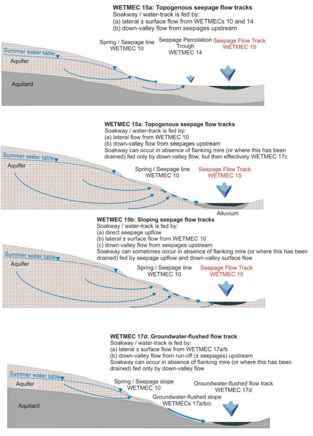
Figure 3.29 Schematic sections of types of Seepage Flow Tracks (WETMEC 15).
