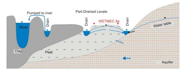
Figure 3.17 Schematic sections of Groundwater-Fed Bottoms (WETMEC 9).
