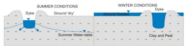
Figure 3.10 Schematic sections of Summer 'Dry' Floodplains (WETMEC 5).
