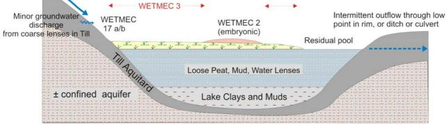
Figure 3.6 Schematic sections of Buoyant, weakly-minerotrophic, topogenous surfaces (WETMEC 3).
