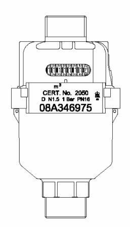
Figure 46 Alternative positioning of m<sup>3</sup> symbol
