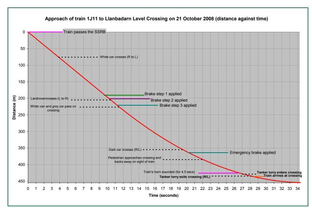
Figure 11: Distance / time plot of the deceleration of the train
