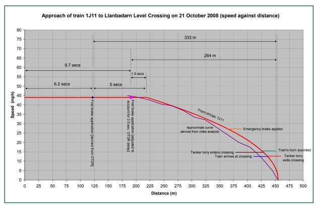
*Figure 12: Speed / distance plot of the deceleration of the train*
