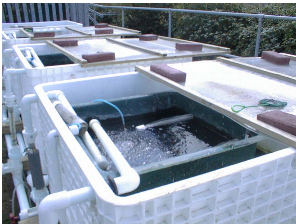
Plate 2. Hatching tanks for roach. To allow monitoring of the developing roach embryos, smaller glass reinforced plastic tanks were fitted into the large mesocosm system tanks. Outflow from these tanks was filtered through fine stainless steel mesh cylinders to prevent loss of fry. Fertilized eggs were placed into mesh hatching trays which were raised above the bottom of the tank to prevent settlement of sediment on the eggs.
