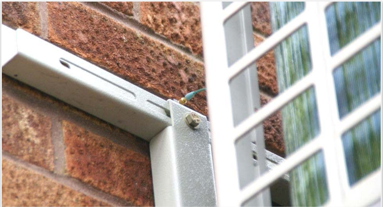
Picture 5-2. 486 Stroud, Wall-mounted Accelerometer
