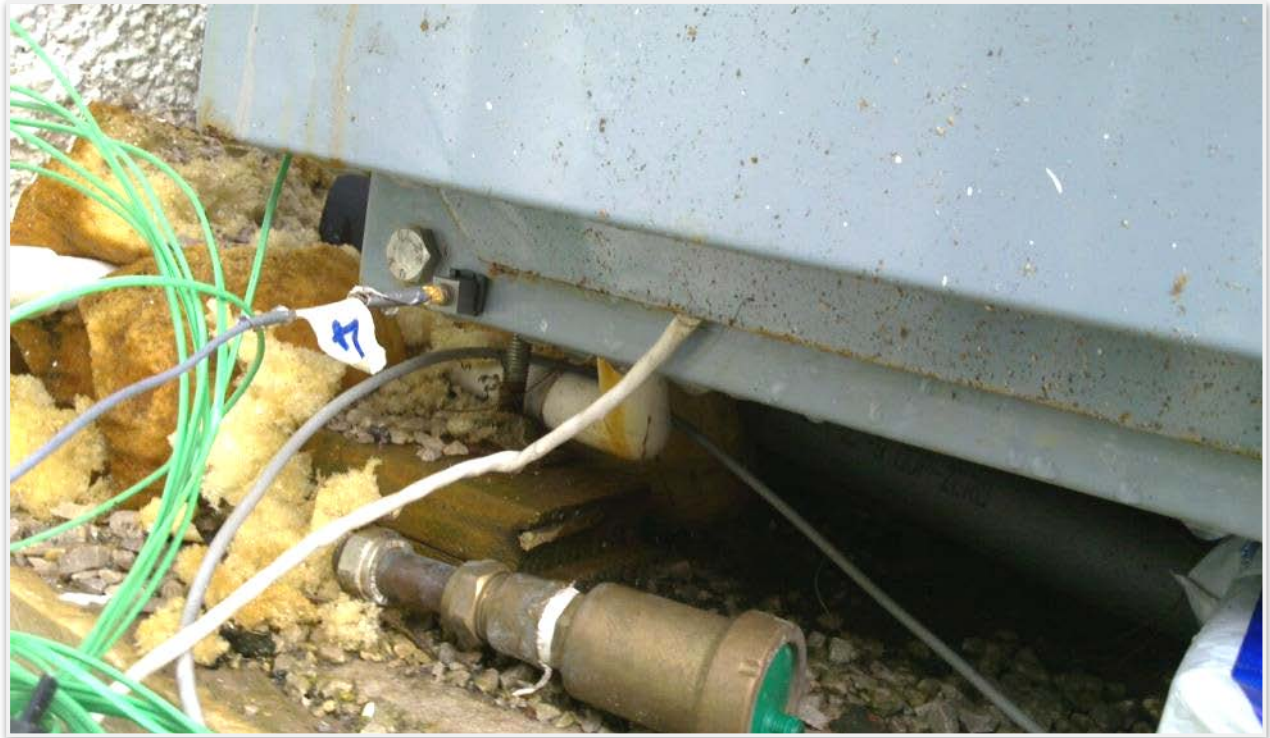
Picture 5-5. 440 Fylde, Casing-mounted Accelerometer
