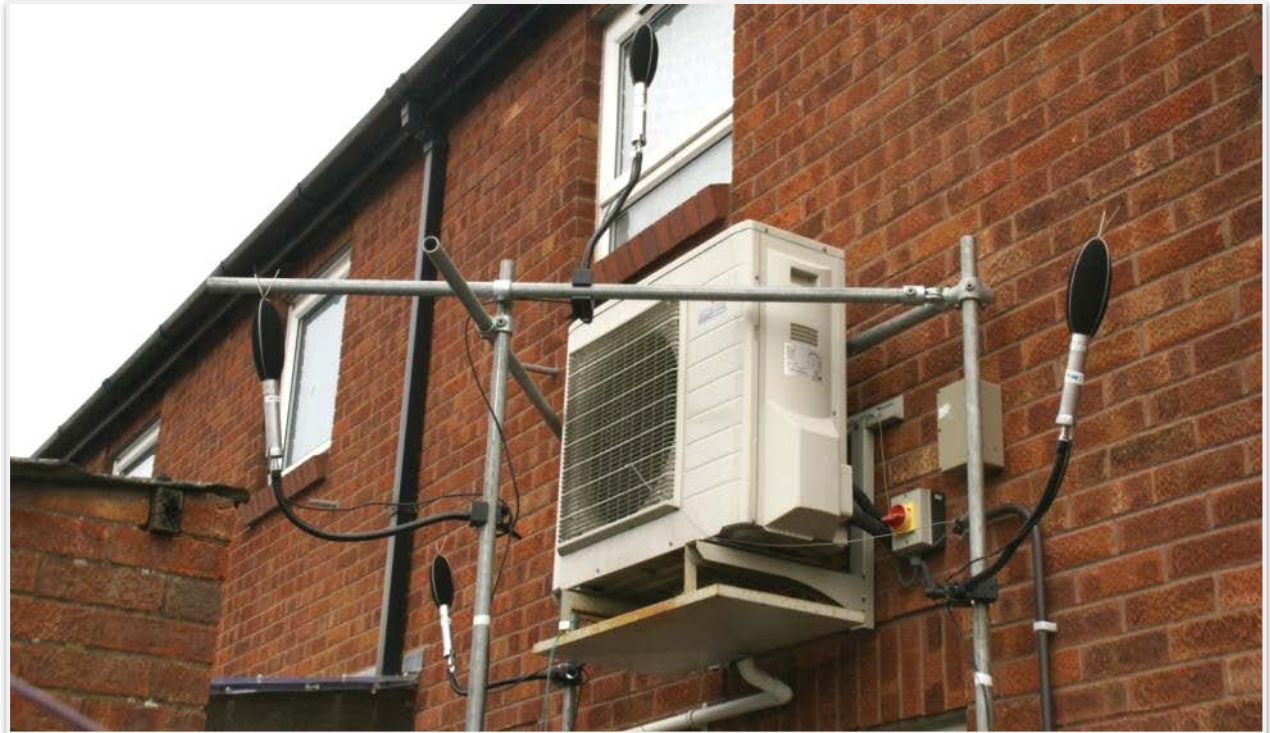
Picture 5-3. 486 Stroud, ASHP and Microphone Arrangement
