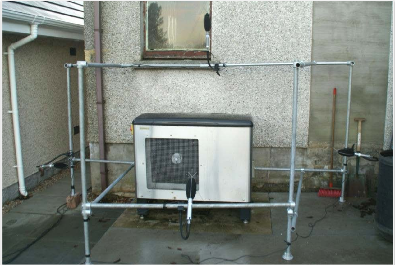
Picture 5-9. 418 Central Buchan, ASHP and Microphone Arrangement
