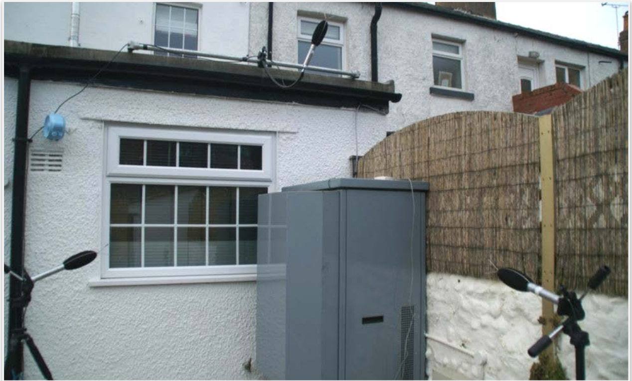
Picture 5-6. 440 Fylde, ASHP and Microphone Arrangement
