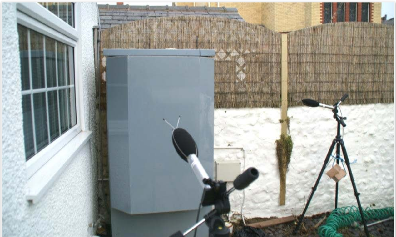
Picture 5-7. 440 Fylde, ASHP and Microphone Arrangement
