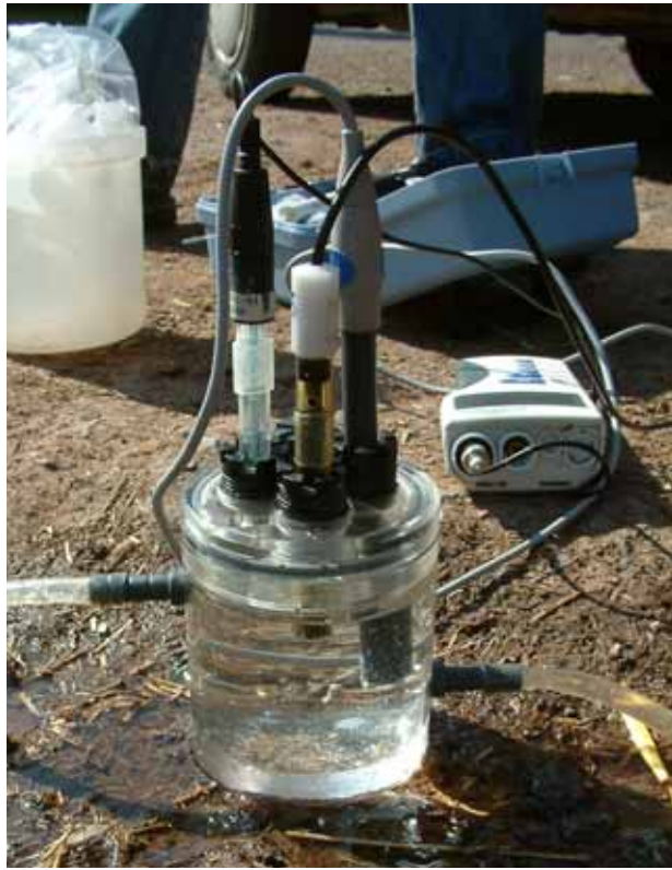
Figure 4.3 Measuring pH, DO and Eh in a flow-through cell.
