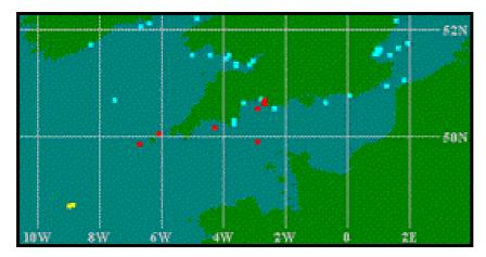
Map 1b Locations for Wave Data Recorders. blue markers indicate short term wave statistics; yellow markers indicate directional wave spectra; red markers indicate one dimentional wave spectra (from British Oceanographic Data Centre)
