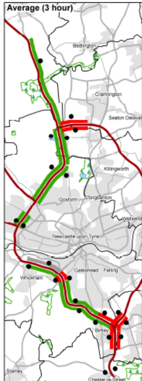
Figure 3.2 Recorded weekday evening peak network flow changes, compared to TEMPRO trip end forecasts
