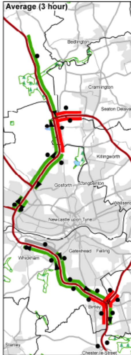
Figure 3.1 Recorded weekday morning peak network flow changes, compared to TEMPRO trip end forecasts
