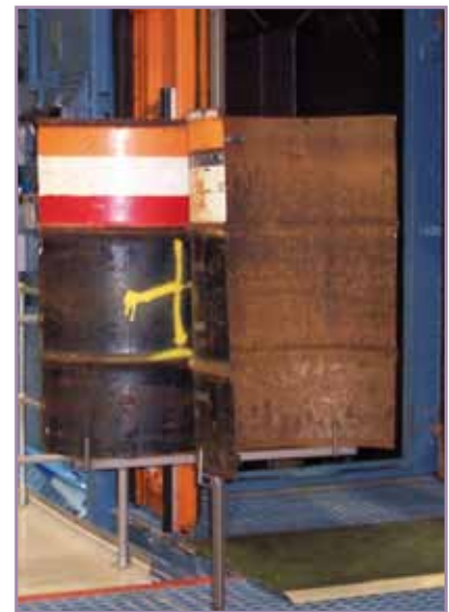
Drums before and after decontamination, after which the metal can be recycled
