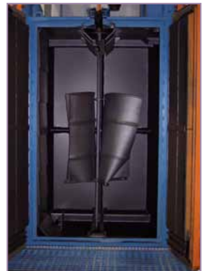
Drums before and after decontamination, after which the metal can be recycled
