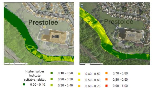
Figure 4.19 shows a substantial decrease in cyprinid 0+ habitat as expected for the returning flowing water conditions. Before weir removal, the best 0+ cyprinid habitat was found upstream of the weir in the impounded backwater. Following weir removal, the increased velocities in what used to be a backwater are less suitable for 0+ cyprinids, while the habitat downstream of the weir remains unsuitable.
