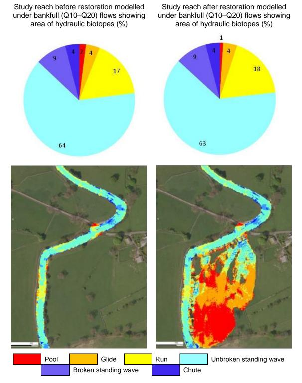
The hydraulic habitat analysis demonstrated that there would be little change following removal of the embankment. In this scenario the channel remains constrained by bank protection. Leaving the channel constricted means that geomorphological processes would be restricted, limiting the effectiveness of any geomorphic recovery from
