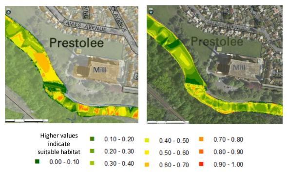
Both before and after weir removal, refugia habitat was available at the margins of the channel and immediately downstream of the weir on the left hand bank (Figure C.10). There was little change in the availability of refugia as a result of the weir's removal.
