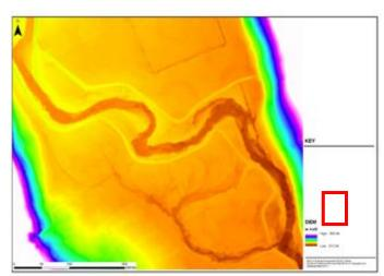
Figure B.1 Example of a DEM model
