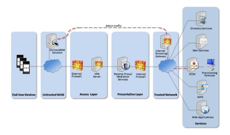
Recommended network architecture for Windows Phone 8.1 deployments using an online MDM solution
