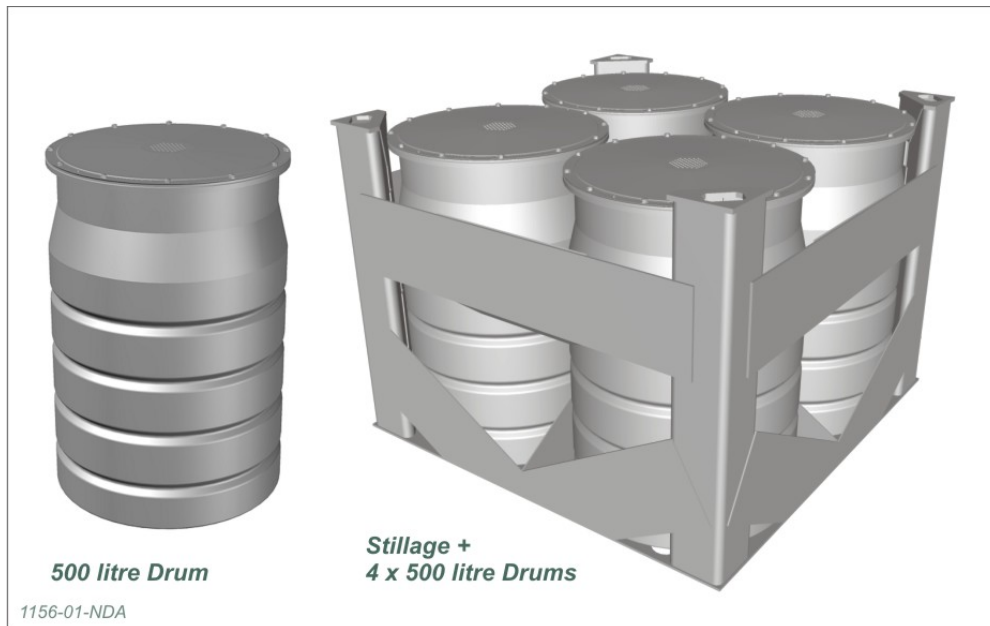
Figure A2 500 litre drums showing vents in the lids [9]
