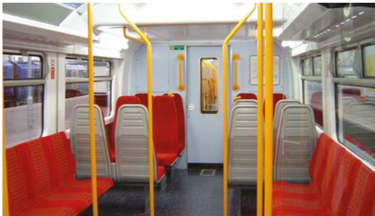
An example of an alternative seating layout to 3 + 2 which provides wider aisles and more comfortable standing space.
