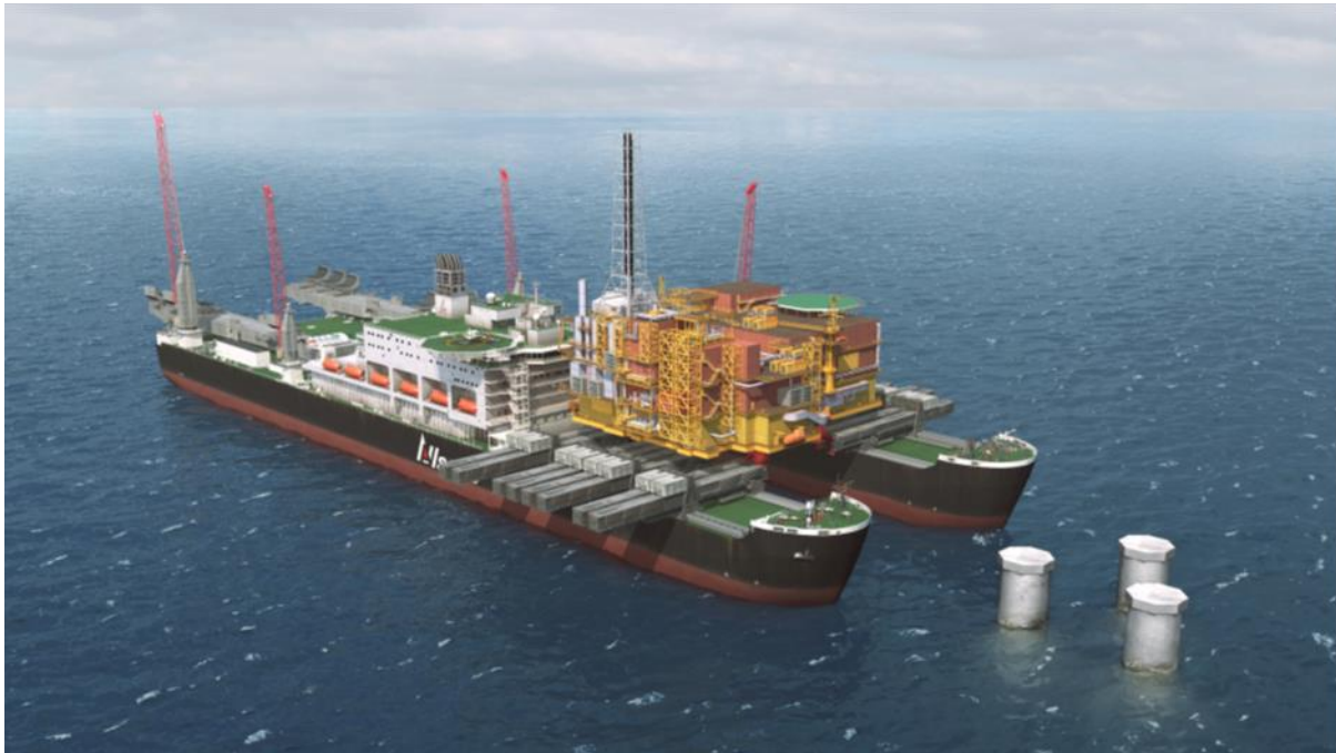
Figure 4.6 The Brent Delta topside secured on the SLV Pioneering Spirit ready for transportation to the nearshore transfer site.
