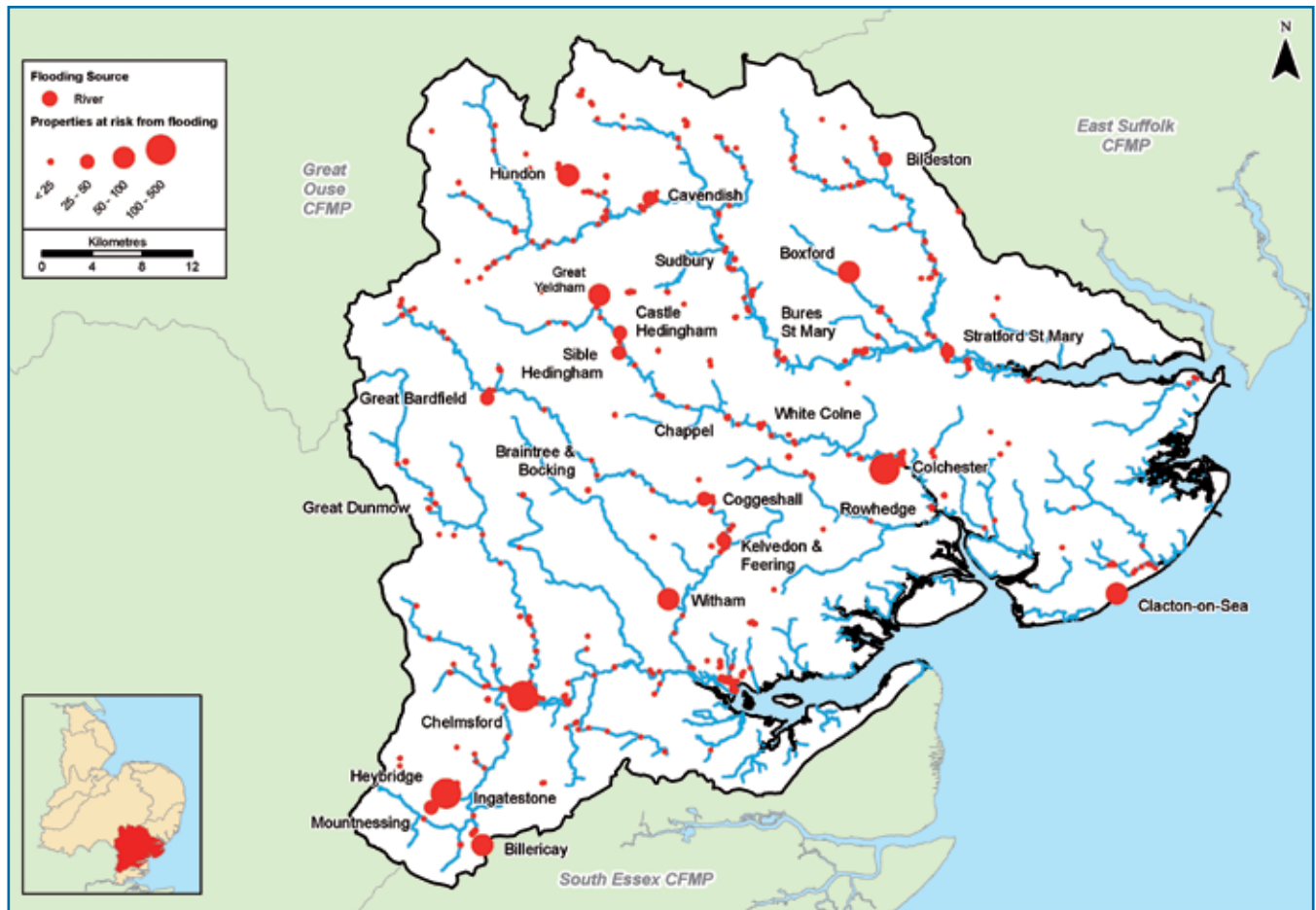
Map 2 Flood risk to property in a 1% annual probability river flood, taking into account current flood defences
